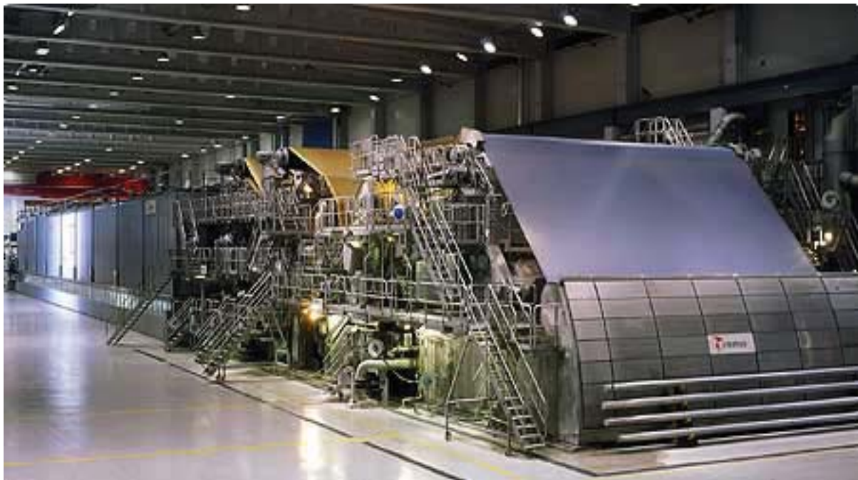
Figure 2. A typical paper machine, To the Courtesy of the Stora Enso Corporation is a Finnish conglomerate; and it is their News Print paper machine at Langerbrugge; Paper Machine Number 4. This machine was built by the Metso Paper Machine Building Group is also from Finland.
