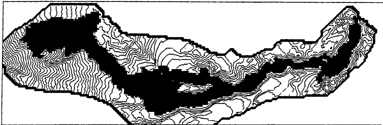
Fig.7: The Mount Ontake landslide simulation with SCIDDICA
