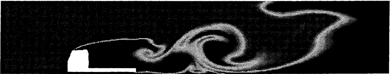
Figure 5. Air flow around a driving Volvo FH truck. Geometry: Courtesy of Volvo Truck Corporation.
