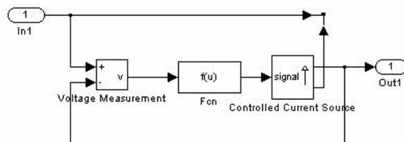
Fig. 3 Simulation model of the voltage controlled current source ( $G_p$ ).
