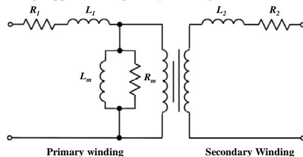
Fig. 4 Transformer model.
