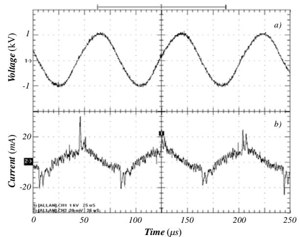
Fig. 6 Experimental results from the reactor (12.5 kHz frequency, transformer primary 75V/9A) a) applied voltage  $V_s(t)$ , b) discharge current.
