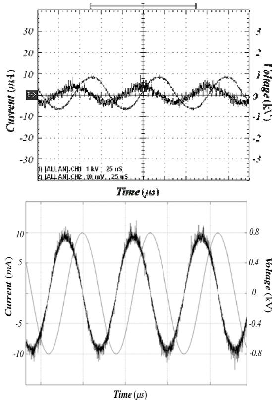
Fig. 7. Comparison of experimental (top) and simulation (bottom) results at 12.5 kHz. The parameters of the voltage transformer primary side are 35V/6A, with  $\alpha=9$ .
