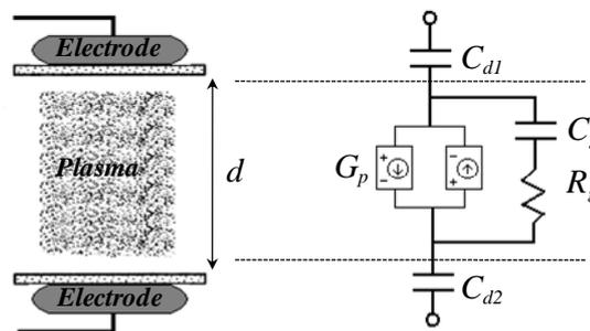
Fig. 1 The DBD cell (left) and its electrical model (right)
