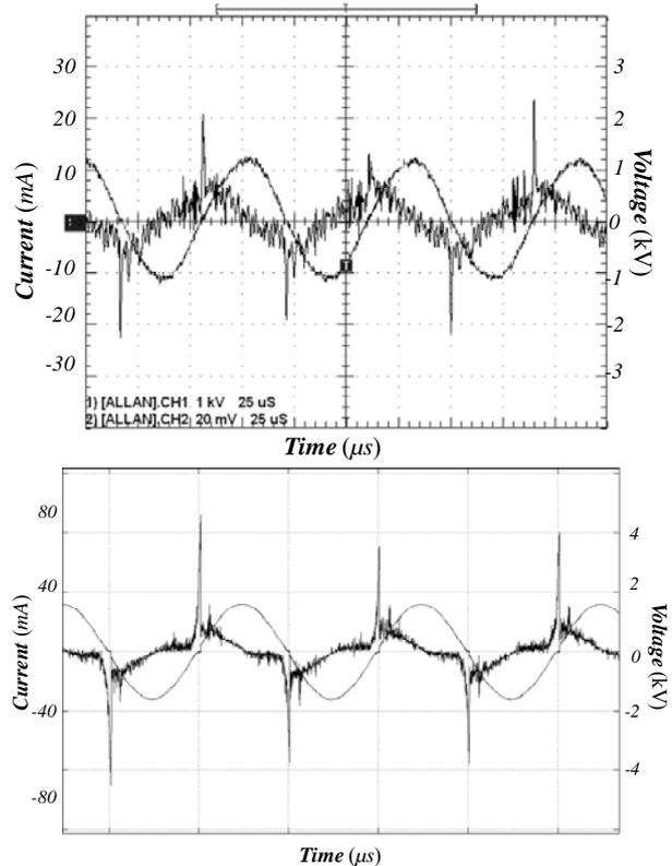
Fig. 9 Comparison of experimental (top) and simulation (bottom) results at 12.5 kHz. The parameters of the voltage transformer primary side are 110V/9A; the coefficient  $\alpha=9$
