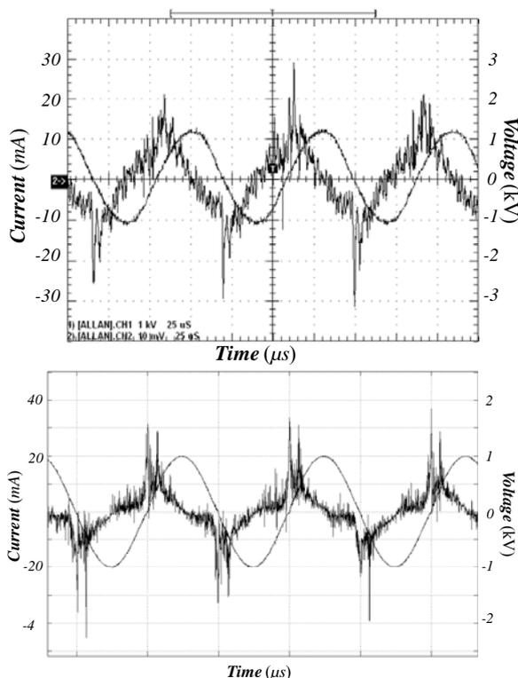
Fig. 8 Comparison of experimental (top) and simulation (bottom) results at 12.5 kHz. The parameters of the voltage transformer primary side are 70V/8A with  $\alpha=9$ .
