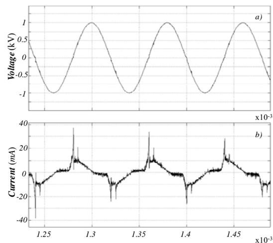
Fig. 5 Simulation results (frequency 12.5 kHz,  $\alpha=12$ ): a) applied voltage  $V_s(t)$ , b) discharge current.
