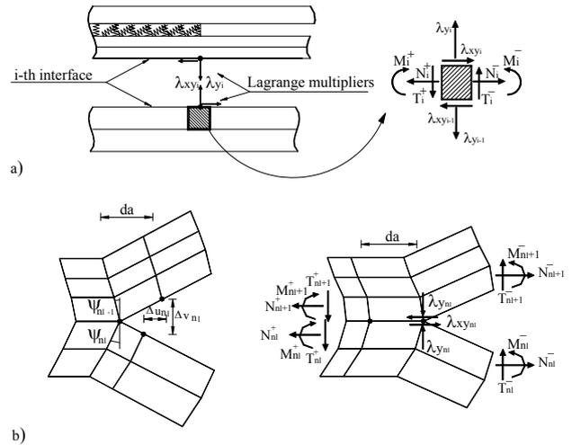
Fig.3 a) Lagrangian forces at the crack tip front. b) Virtual crack closure methods.
