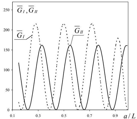
Fig.14 Dimensionless ERR mode components as a function of the crack extension:  $c/c_{sh}=0.6$
