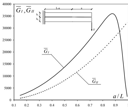
Fig.12 Dimensionless ERR mode components as a function of the crack extension:  $c/c_{sh}=0$ , static case.
