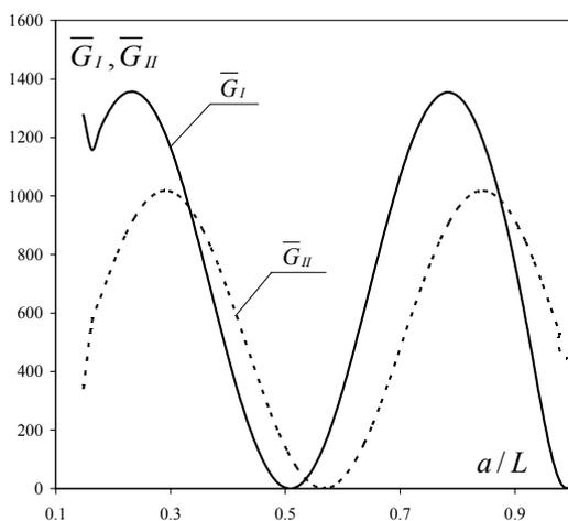
Fig.13 Dimensionless ERR mode components as a function of the crack extension:  $c/c_{sh}=0.3$
