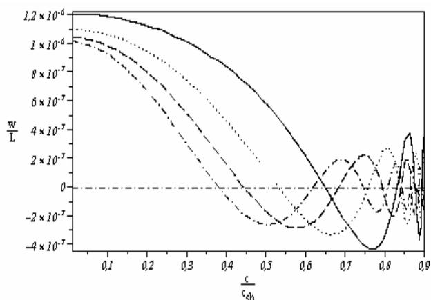
Fig.6 Mode I loading conditions: Dimensionless relative displacements close to the crack tip front.
