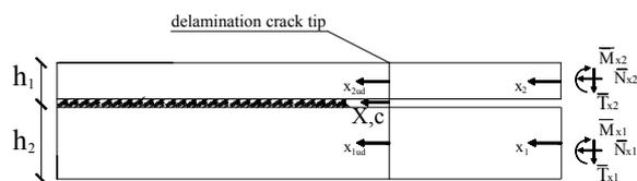
Fig.2 Two layer scheme – Moving and fixed coordinate systems.
