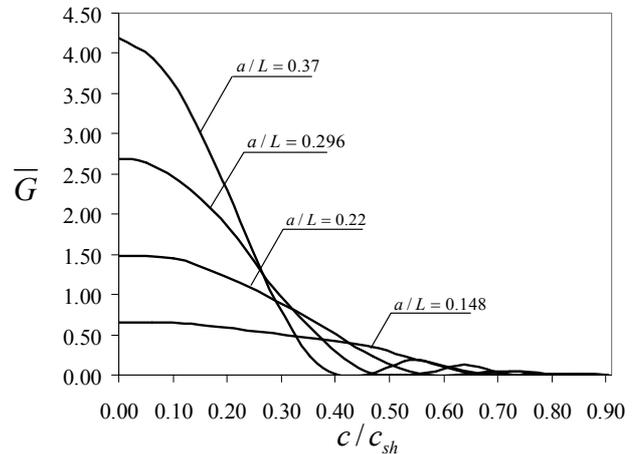
Fig.9 Mode II loading conditions: Dimensionless ERRs for different speed of the crack front.
