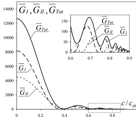
Fig.10 Mixed mode loading conditions: Dimensionless ERRs for different speed of the crack front.
