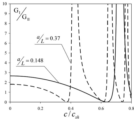
Fig.11: Mode mix ratio versus speed of the crack front.
