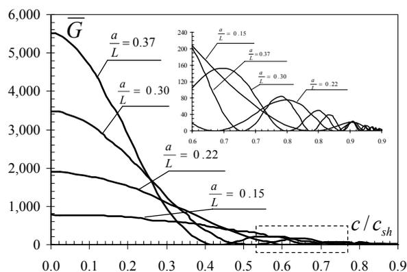
Fig.5 Dimensionless ERR for different speed of the crack front and initial delaminated length..
