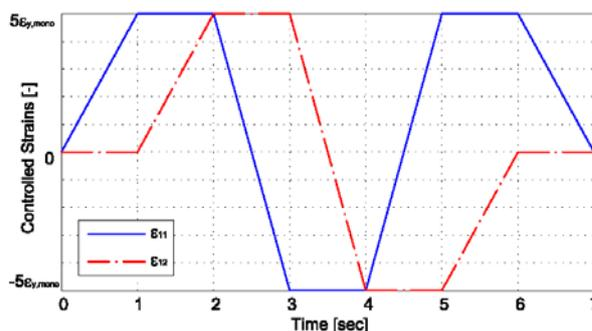
Fig. 1 Mixed stress-strain loading history: time evolution of controlled strains.
