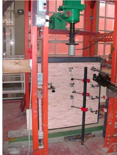
Fig. 3: Steel frame, instrumentation and tested panel.
