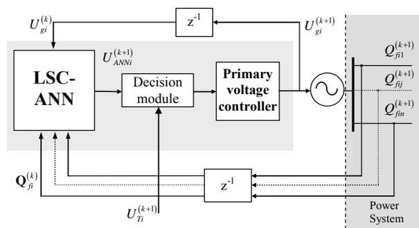
Fig. 1 LSC-ANN control scheme for generator  $i$
