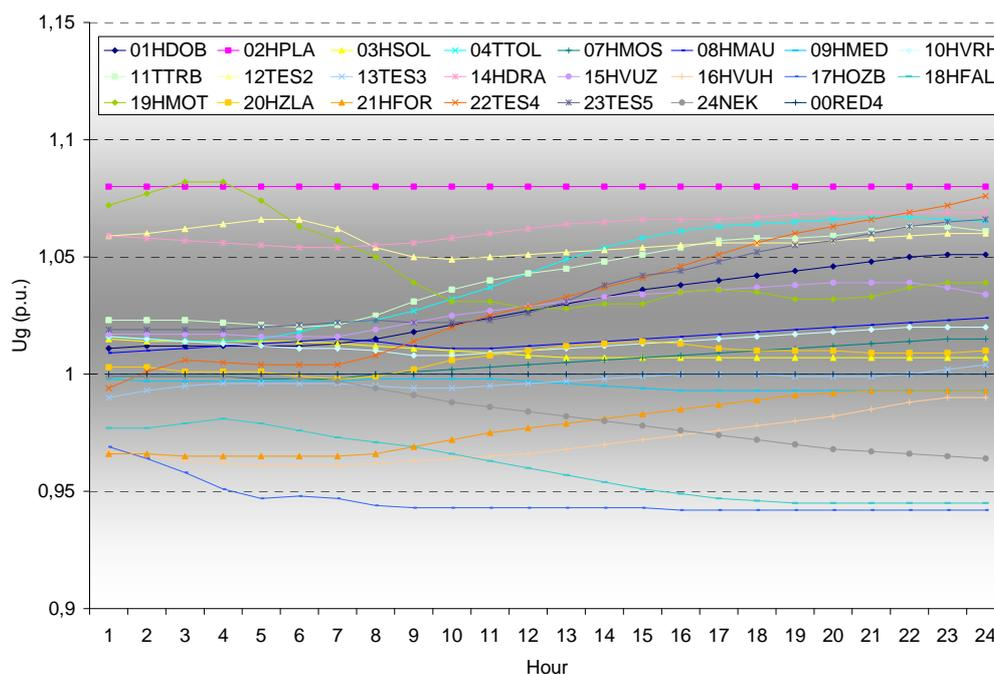
Fig. 6 Generator voltage profile for 24-hour period, ANN control
