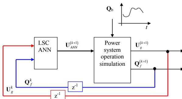
Fig. 2. Discrete simulation loop
