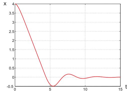
Fig. 9 Transient response (PID)
