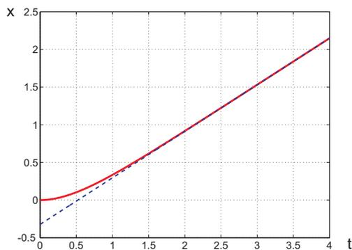
Fig. 8 Step response of the open loop system
