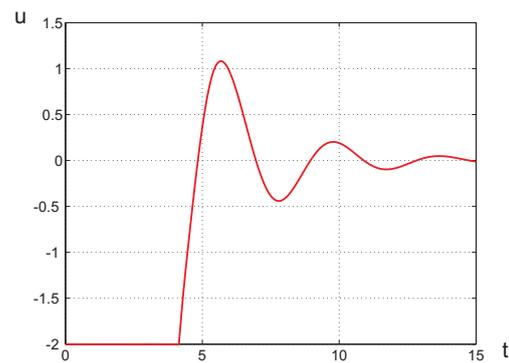
Fig. 10 Control input versus time (PID)
