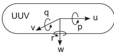
Fig. 3 Definition of body fixed coordinate system
