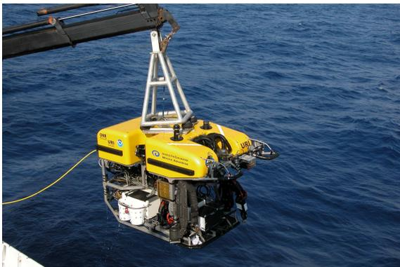
Fig. 1 A science ROV being launched from an oceanographic research vessel [1].
