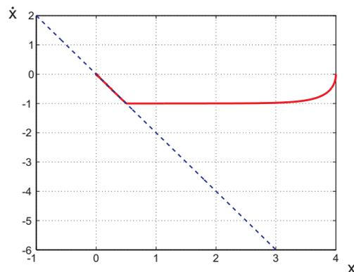
Fig. 5 The phase diagram of transient response (SMC)
