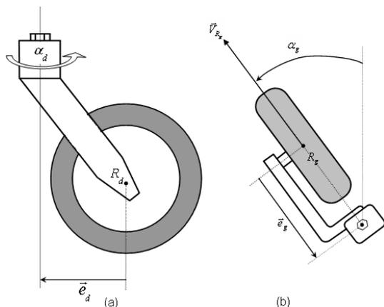
Fig. 2 (a) Schema of the side view of the right front Wheel (b) Schema of the high view of the left front
