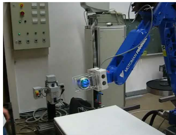
Fig. 10 Experimental systems et up ( Powerball®, sensor griper, and the robot wrist)
