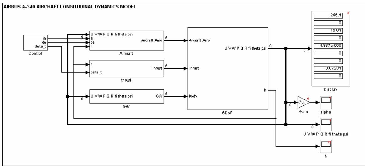
Fig.2 Top view of the Matlab-Simulink block diagram of AIRBUS-A340-300 passenger aircraft
