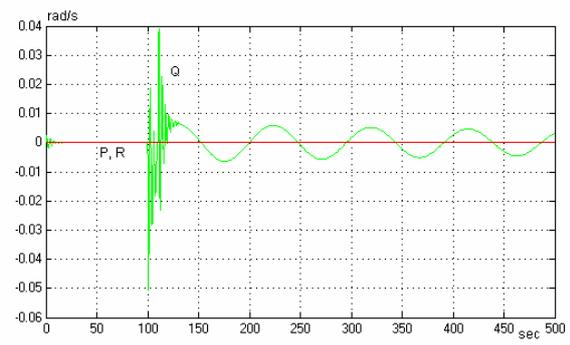
Fig.8 Attitude rates:  $p$ -roll rate  $q$ -pitch rate  $r$ -yaw rate
