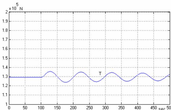
Fig.11 Total thrust produced by 4 turbofan engines
