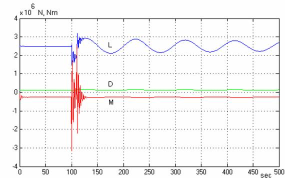
Fig.10 Aerodynamic forces and moments ( $L$ ,  $D$ ,  $M$ )
