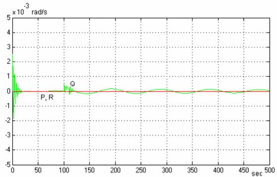
Fig.16 Attitude rates:  $p$ -roll rate  $q$ -pitch rate  $r$ -yaw rate
