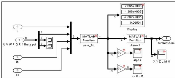
Fig.3 Block diagram of aircraft block-set
