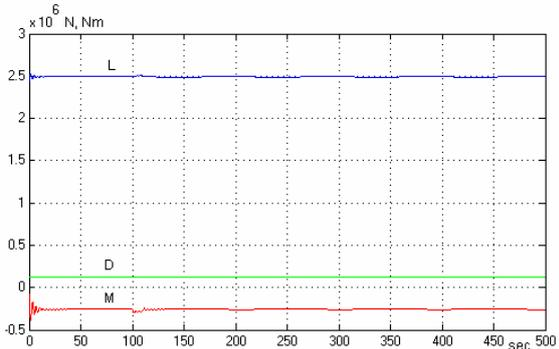
Fig.18 Aerodynamic forces and moments ( $L$ ,  $D$ ,  $M$ )
