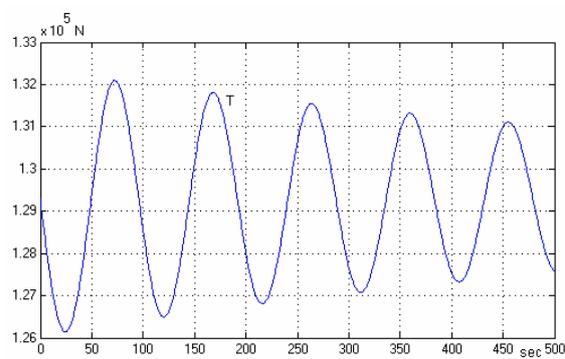
Fig.27 Total thrust produced by 4 turbofan engines
