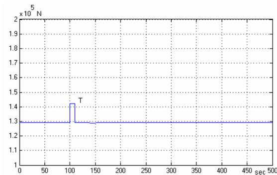
Fig.19 Total thrust produced by 4 turbofan engines
