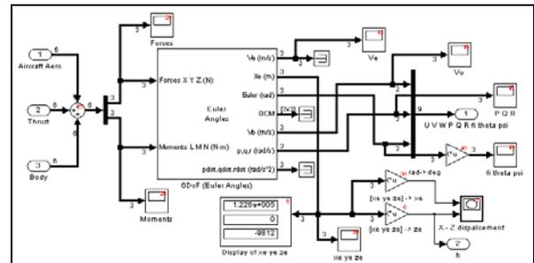
Fig.6 Block diagram of 6DoF block-set.
