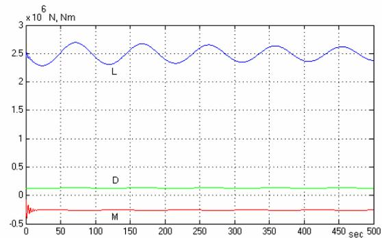
Fig.26 Aerodynamic forces and moments ( $L$ ,  $D$ ,  $M$ )
