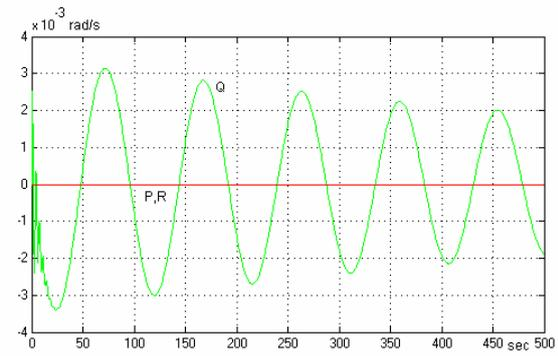
Fig.24 Attitude rates:  $p$ -roll rate  $q$ -pitch rate  $r$ -yaw rate
