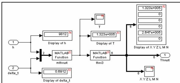
Fig.4 Block diagram of thrust block-set
