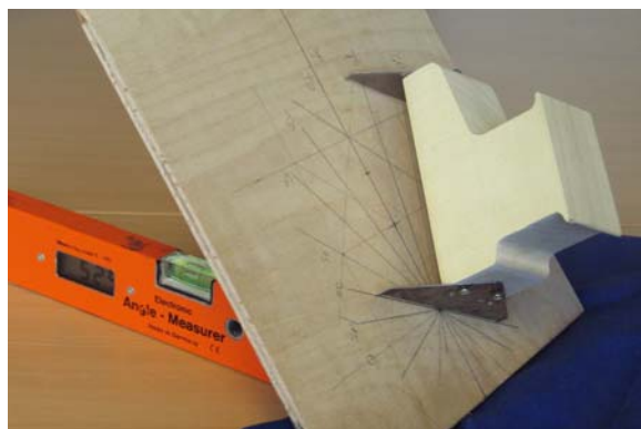
Fig. 14 Measuring static stability of a characteristic model of a tractor in relation to its position on a slope
