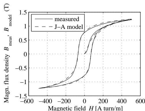
Fig. 3 Measured and calculated hysteresis loops
