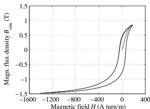
Fig. 9 Calculated B-H hysteresis loop for the case when nonlinear load is used
