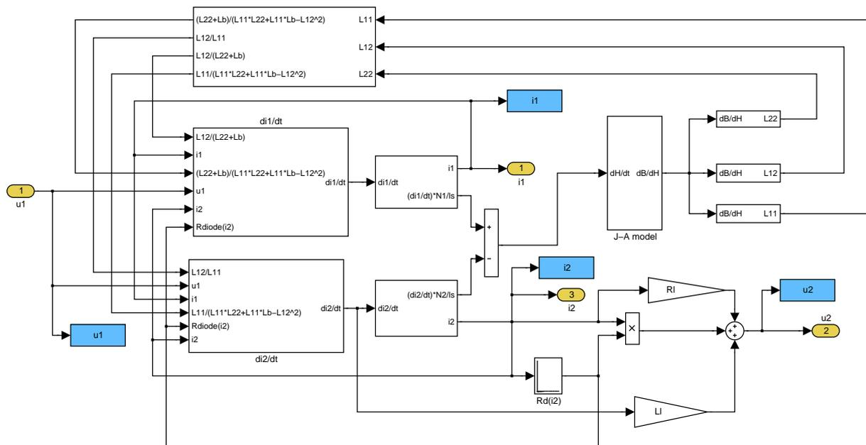
Fig. 1 Block scheme of a nonlinear single phase transformer with nonlinear load
