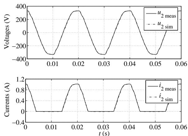
Fig. 8 Measured and calculated secondary voltages and currents when nonlinear load is considered
