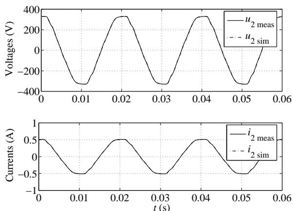
Fig. 5 Measured and calculated secondary voltages and currents when linear load is considered
