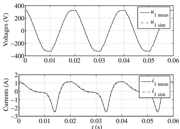
Fig. 7 Measured and calculated primary voltages and currents when nonlinear load is considered
