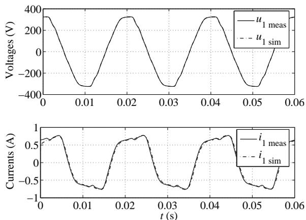
Fig. 4 Measured and calculated primary voltages and currents when linear load is considered
