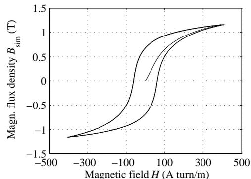
Fig. 6 Calculated  $B - H$  hysteresis loop for the case when linear load is used
