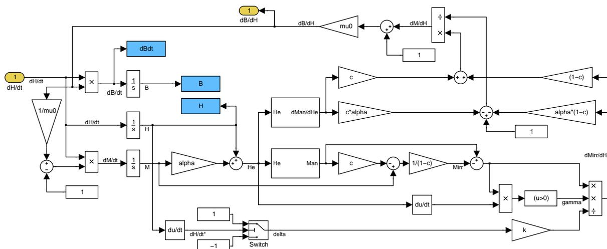
Fig. 2 Block scheme of the J-A hysteresis model
