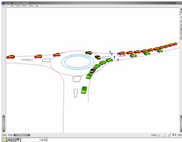
Fig. 4 Microsimulation model of roundabout–detail I
