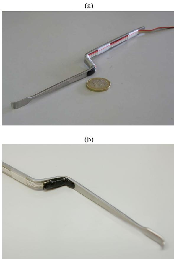
Fig. 6 Two prototype retractor for force measurement. Piezoresistors are covered with black epoxy cast. (a) Sensors bonded on back side. (b) Sensors bonded on front side.
