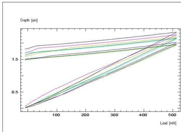
Fig. 4 Depth–load diagram determined by the indentation method. (From the slopes of the curves and starting and ending load point the Young's modulus is calculated by the method described in [9].)
