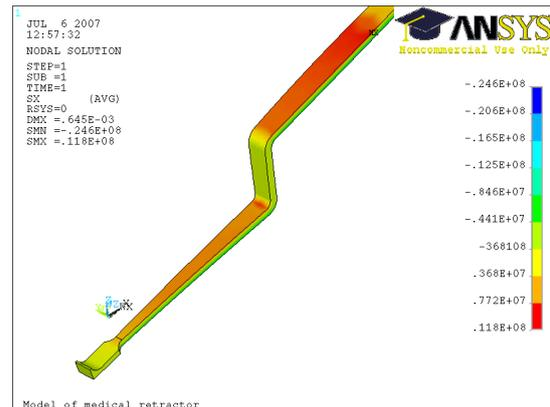
Fig. 5 Stresses in longitudinal ( $x$ ) direction in loaded retractor.
