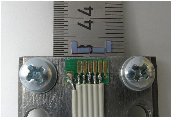
Fig. 3 Stainless steel cantilever with four piezoresistors prepared to operate in bridge circuit.
