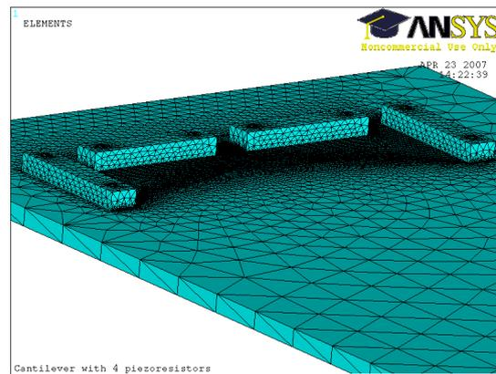
Fig. 1 Meshed model of piezoresistor chips on stainless steel cantilever used to determine coefficients that build up  $[\pi]$  matrix. Due to the symmetry only half of the model must actually be solved.
