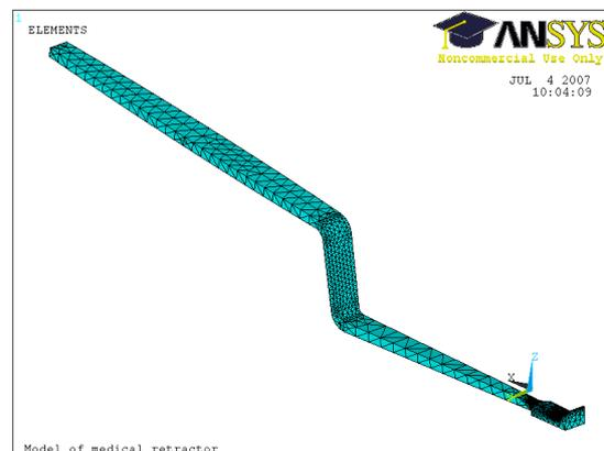
Fig. 2 Meshed model of medical retractor. Stresses in the retractor are important for piezoresistor placement.
