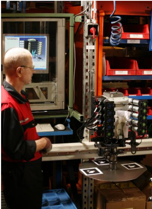
Figure 8 Industrial pilot case (Courtesy of Valtra Plc). The round plate includes the markers to track the orientation of the hydraulic block.
