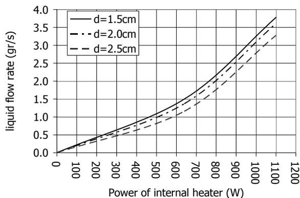
Figure 5. Variation of liquid Flow rate versus internal heater power (external heat power = 600 W)
