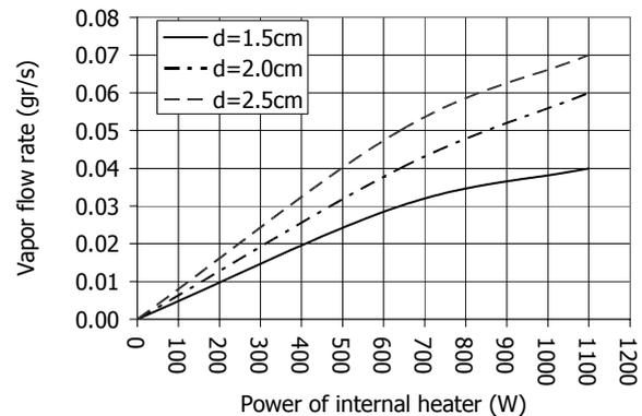
Figure 2. Variation of vapor Flow rate versus internal heat power (external heat power = 300 W)
