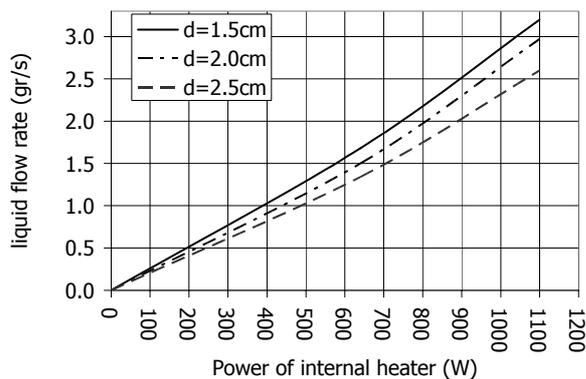
Figure 4. Liquid Flow rate versus internal heat power (external heat power = 300 W)
