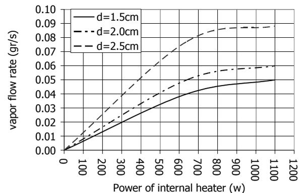
Figure 3. Variation of vapor Flow rate versus internal heat power (external heat power = 600 W)
