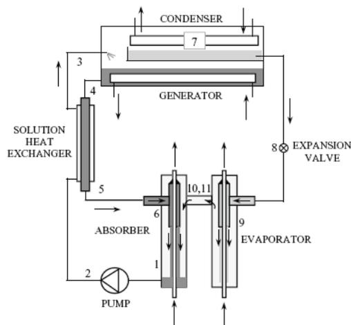
Figure 7. A schematic of a LiBr Absorption system
