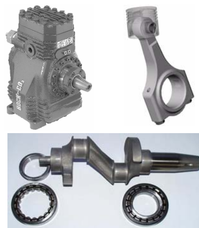
Fig. 1 Mechanical parts of the CO 2 compressor used in prototype AC systems for busses
