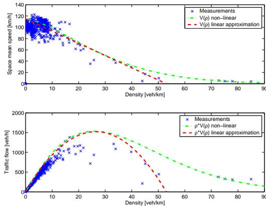
Fig. 2 The theoretical and the fitted fundamental relationship
