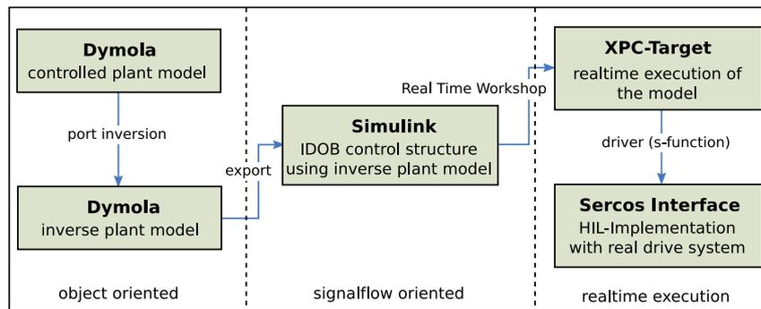
Fig. 7 Tool based IDOB implementation workflow.
