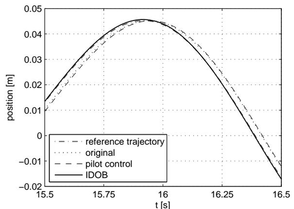
Fig. 10 Comparison of original and IDOB tracking.
