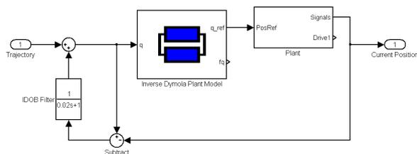
Fig. 9 IDOB structure as Simulink model.
