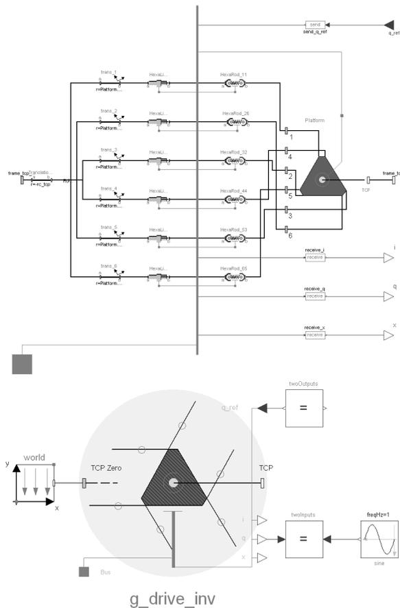
Fig. 4 Inversion example of the overall PKM model; top: plant model, bottom: formation of the inverse system.
