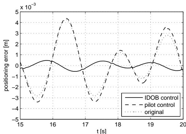
Fig. 11 Comparison of original and IDOB tracking errors.
