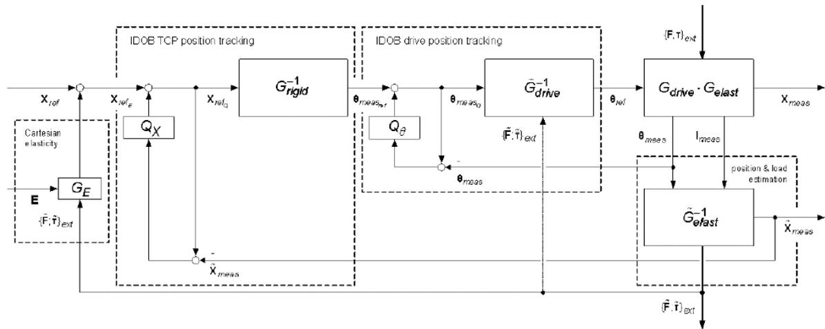
Fig. 2 Cascaded IDOB control scheme of multi axes system
