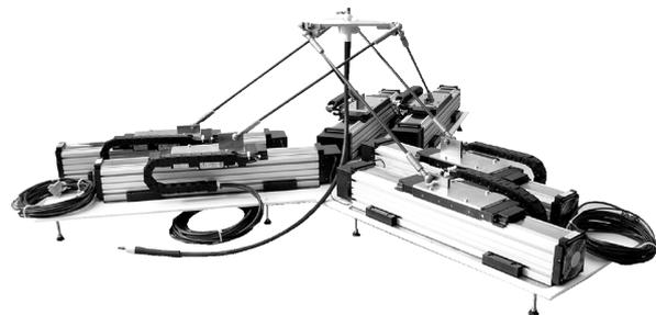
Fig. 3 Parallel kinematic machine *Black Beetle*
