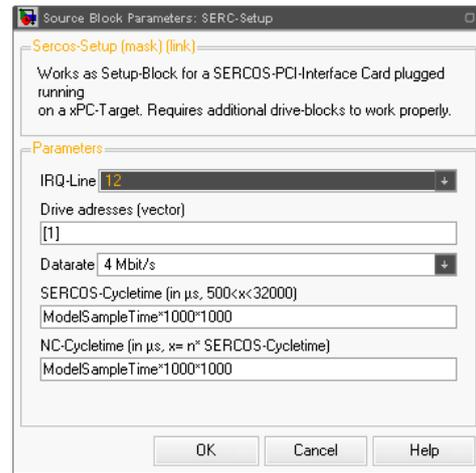
Fig. 5 Bus configuration dialog of the Sercos-Interface blockset for simulink.
