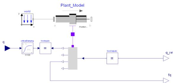
Fig. 8 Inverse Dymola plant model  $\tilde{G}_{drive}^{-1}$  (one axis drive).
