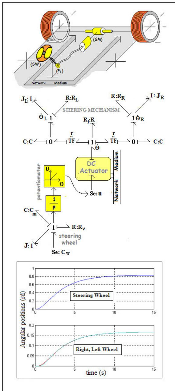
Fig. 7 : Models of the electric steering device
