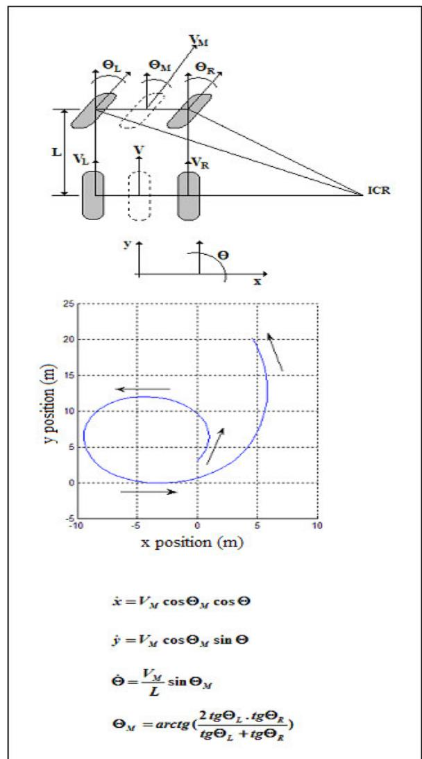
Fig. 2 Two wheels model for car steering
