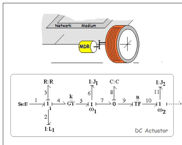
Fig. 3 Model Bond Graph of the main actuator (DC motor)
