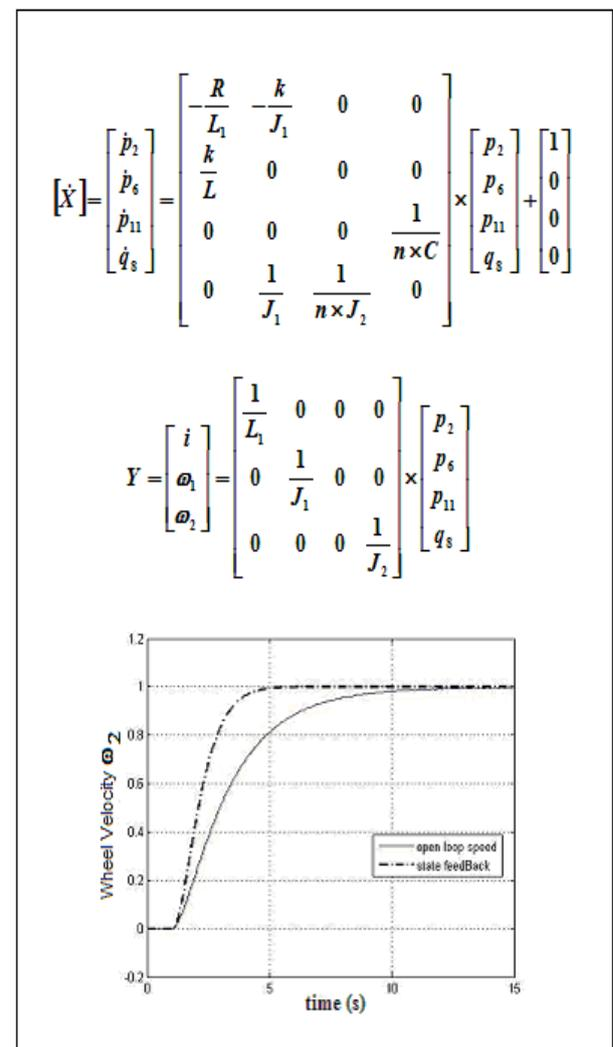
Fig. 4 State Space model and simulation results (velocity  $w_2$ )
