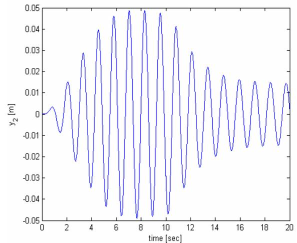
Fig. 6 Displacement  $y_2$  of the absorber after starting (10 sec) the LQR control (alt. 1)
