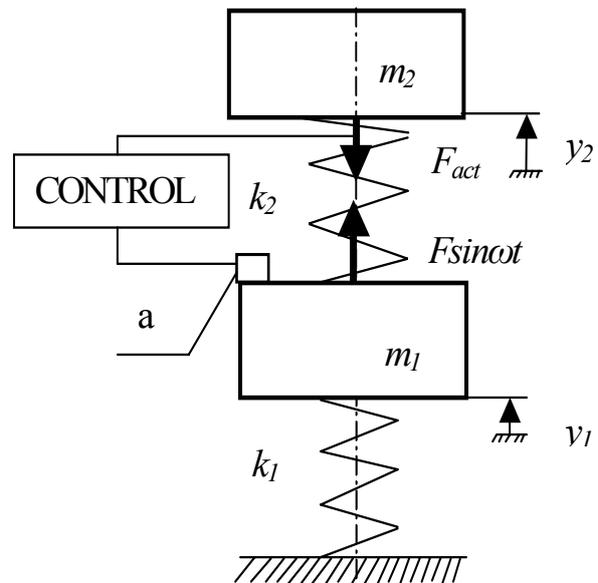
Fig. 1 The model of the mechanical system with an affiliate control absorber  $m_2$
