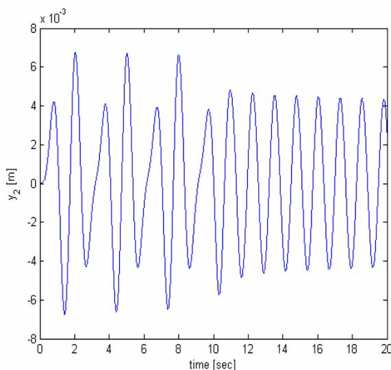
Fig. 10 Displacement  $y_2$  of the absorber after starting (10 sec) the LQR control (alt. 3)
