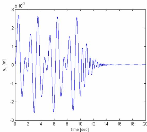
Fig. 9 Displacement  $y_1$  of the system after starting (10 sec) the LQR control (alt. 3)
