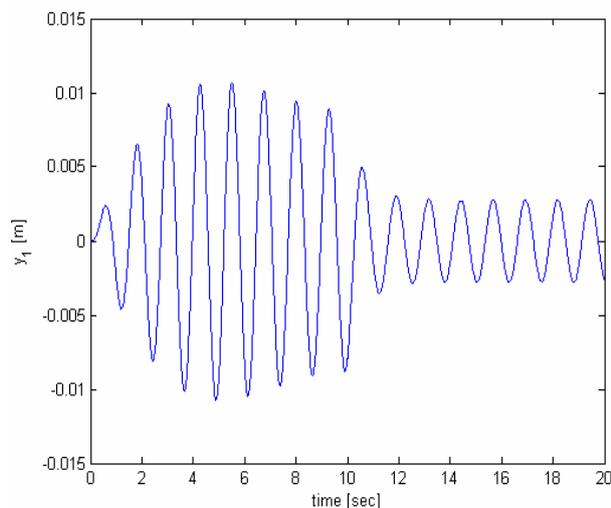
Fig. 5 Displacement  $y_1$  of the mechanical system after starting (10 sec) the LQR control (alt. 1)
