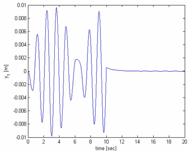
Fig. 7 Displacement  $y_1$  of the mechanical system after starting (10 sec) the LQR control (alt. 2)
