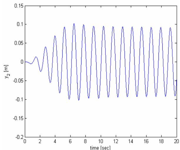
Fig. 8 Displacement  $y_2$  of the absorber after starting (10 sec) the LQR control (alt. 1)
