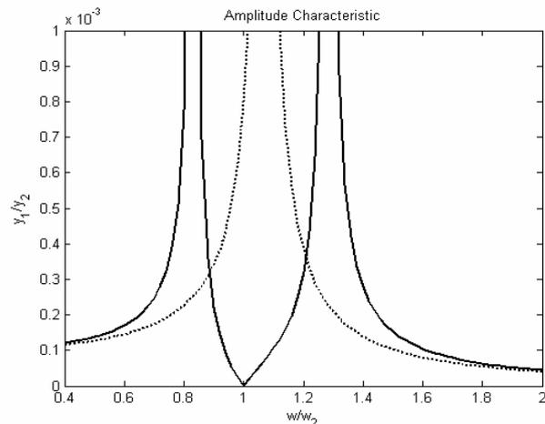
Fig. 2 The amplitude characteristic compared to dimensionless variables (the dotted line is without the absorber)
