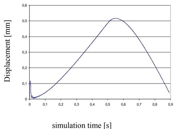
Fig. 10: Dynamic displacement of the laser interferometer measuring point at the mirror
