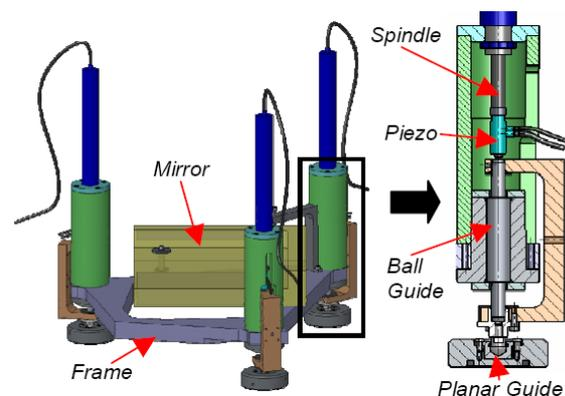
Fig. 2: Model of the vertical axis with spindle and piezo drives [1]
