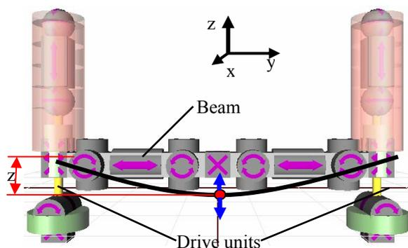
Fig. 3: MBS-model of the reduced vertical axis
