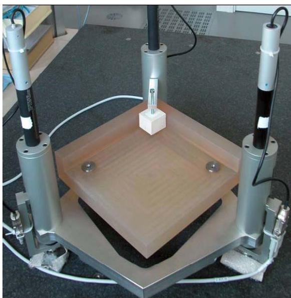
Fig. 1: Design of the vertical axis with mirror
