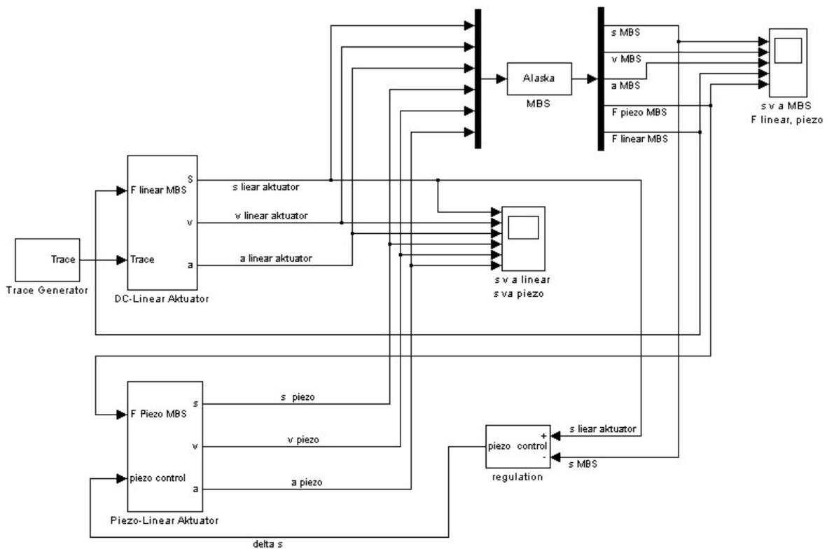
Fig. 6: Simulink block diagram of the vertical axis
