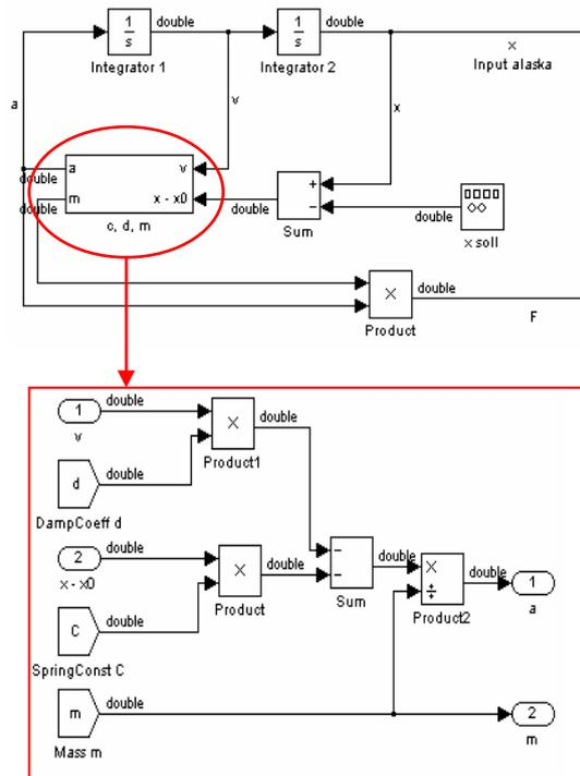
Fig. 5: Simulink model of the piezo drive
