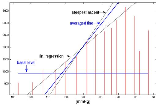
Fig. 3: Determination of the systolic blood pressure
