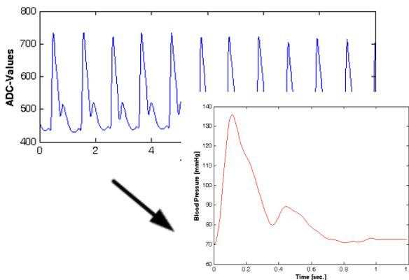
Fig. 4: Sampled Pulse wave
