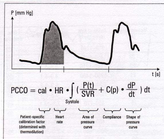
Fig. 2: Example for a pulse contour analysis method - PICCO by PULSION Medical Systems AG
