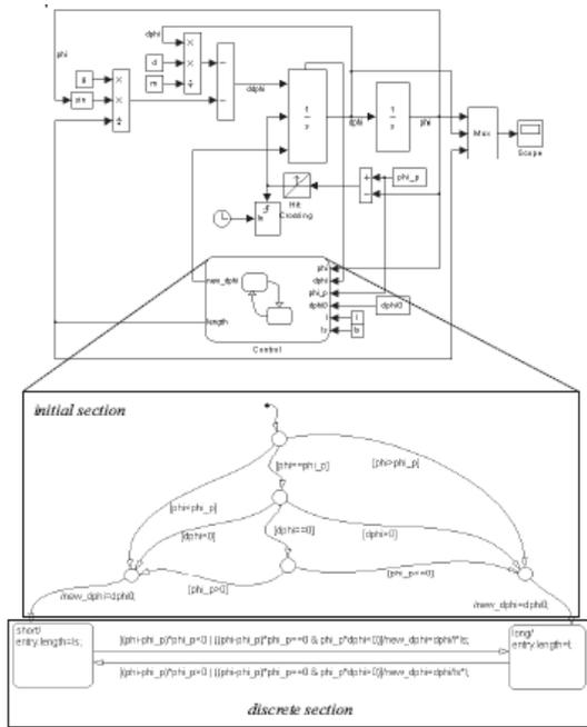
Fig.15 Simulink model for *Constrained Pendulum* with external event detected by hit-crossing block and controlled by Stateflow
