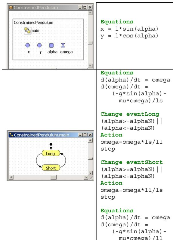
Fig. 18 AnyLogic model for *Constrained Pendulum*, hybrid model decomposition with two pendulum models and *external event*
