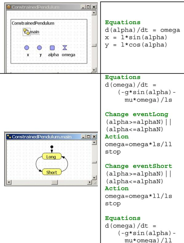
Fig. 19 AnyLogic model for *Constrained Pendulum*, hybrid model decomposition with two models for angular velocity and overall model for angle, controlled by *external event*
