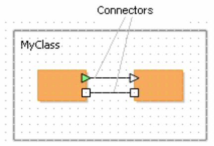
Fig.6 Active objects with connectors exchanging discrete messages (rectangle ports) and continuous signals (triangle ports)
