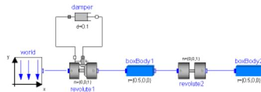
Figure 5 Graphical Modelica model for double pendulum
