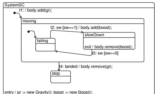
Fig. 17 State chart for dynamics of landing device, Modelica Extension in Mosilab
