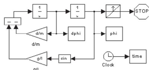
Fig.14 Simulink model for *Constrained Pendulum* with *external* event detected by hit-crossing block
