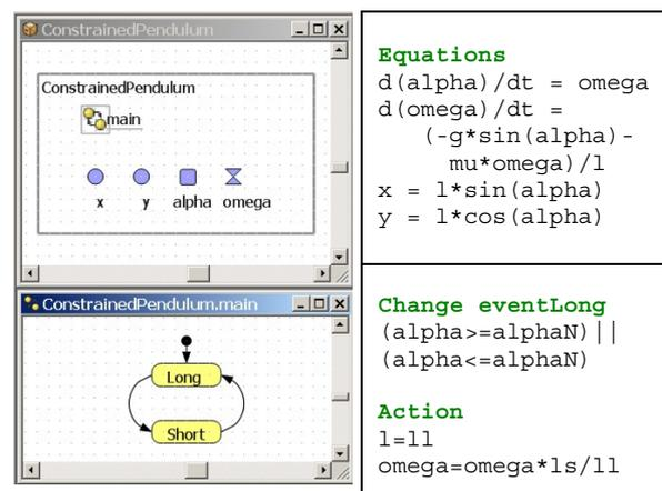
Fig.8 AnyLogic model for *Constrained Pendulum*, simple implementation
