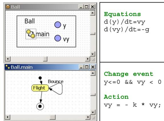
Fig.7 AnyLogic model for the *Bouncing Ball*
