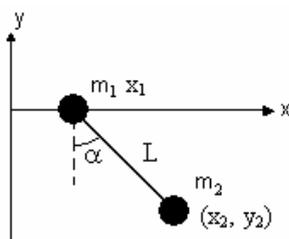
Fig.20 MVS model for pendulum with free suspension – model definition with physical laws (DAEs)
