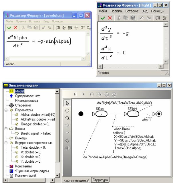
Fig.21 MVS model for breaking pendulum - hybrid model decomposition into pendulum and flight model, controlled by an external event of type E-SE-D
