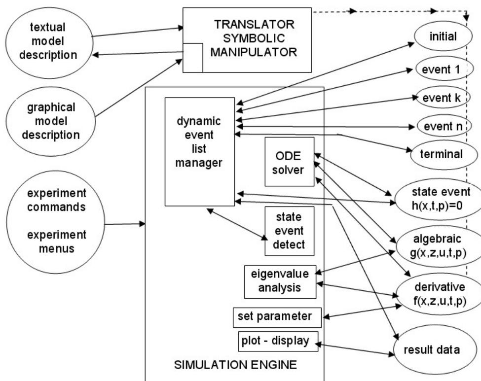
Fig. 2 Extended structure of a simulation system with discrete elements (events)
