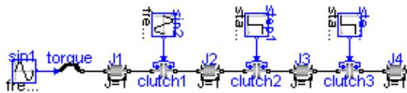
Figure 4 Graphical Modelica model for coupled clutches
