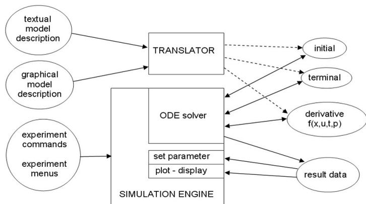
Fig.1 Basic structure of a simulation language due to CSSL standard
