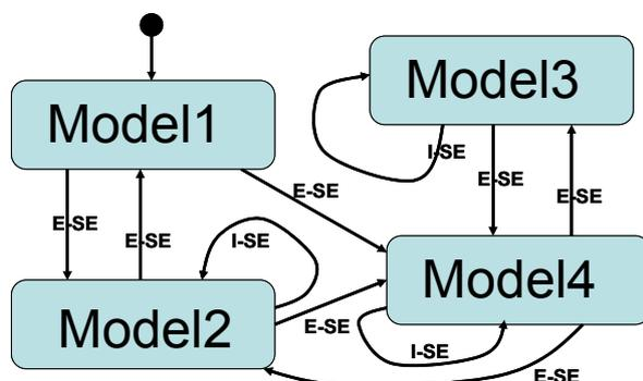
Fig.13 State chart control for different models with *internal* and *external* events
