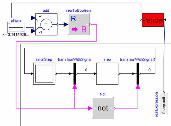
Fig.16 Graphical Dymola model for *Constrained Pendulum* with internal events managed by elements of Dymola's state chart library
