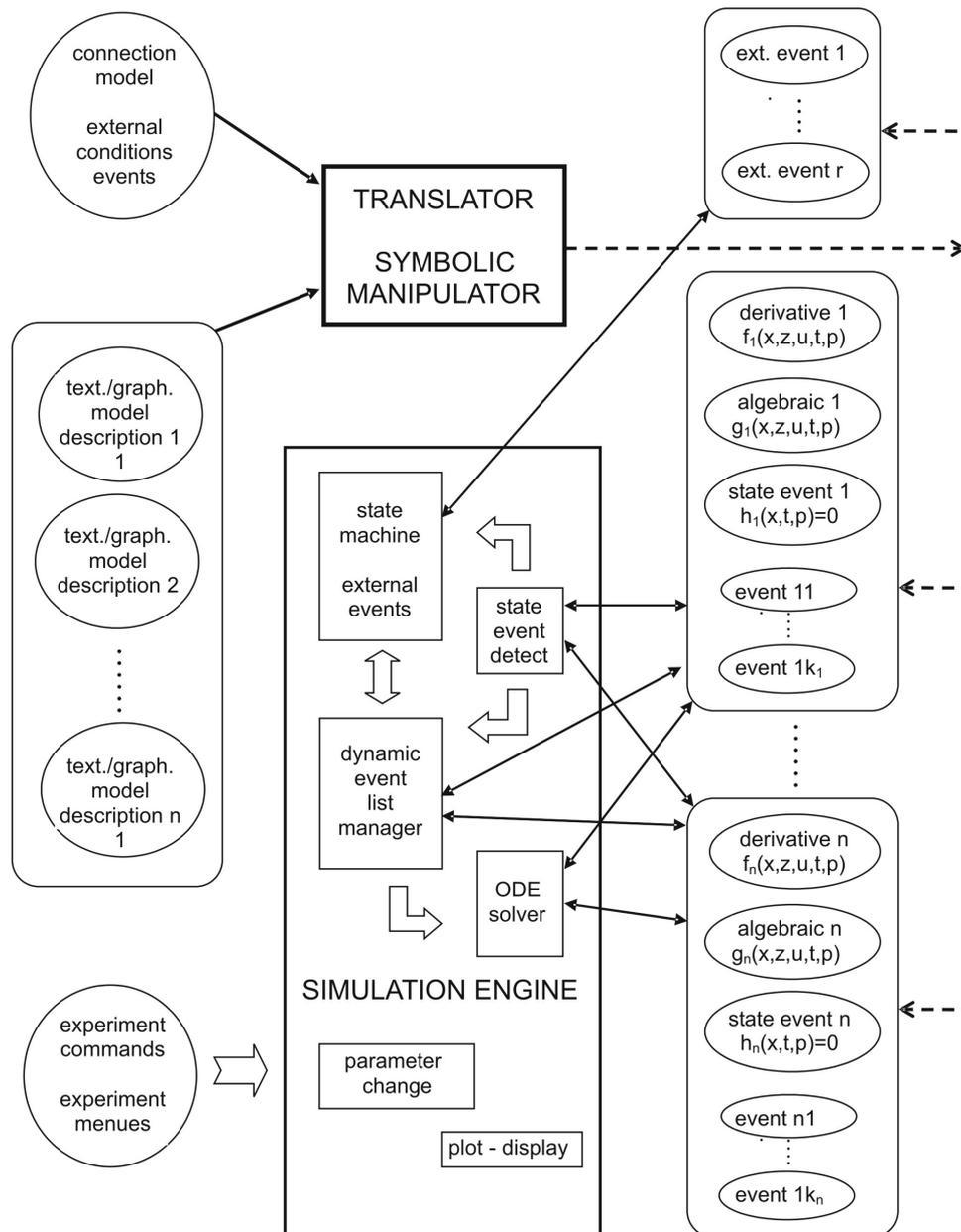
Fig. 12 Structure for a simulation system with *external state events* E-SE and classical internal state events I-SE for controlling different models.
