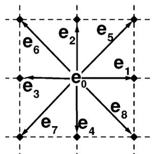
Fig. 5 The VEGF particles move on a cartesian grid with the velocities  $\mathbf{e}_0 \dots \mathbf{e}_8$
