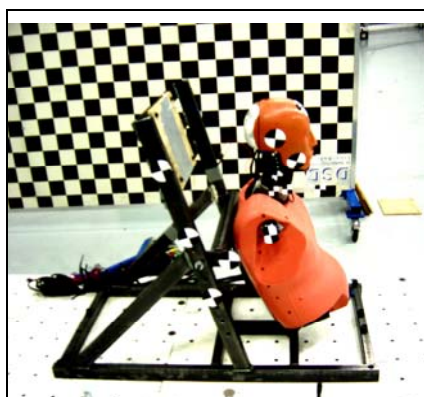
Fig. 8 Rack for component tests with torso
