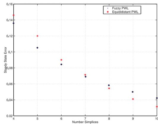
Fig. 6 Steady-State errors using 500 points for several number of simplices.
