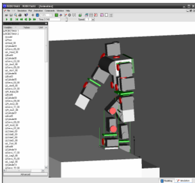
Fig. 6: A screenshot taken in Dymola during simulation of the final motion
