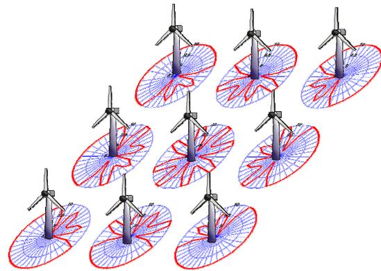
Fig. 7 Wake wind roses for individual WT's and constant input wind speed (10m/s; 0°-360°)
