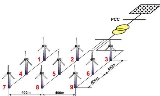
Fig. 6 Structure of the test wind farm
