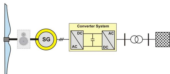
Fig. 2 Structure of the WT with converter facilitated SG
