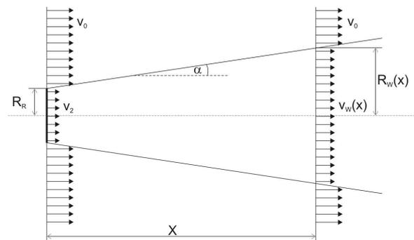
Fig. 4 Structure of the wake model by Jensen
