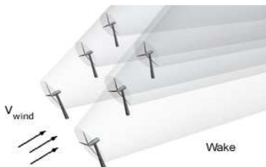
Fig. 3 Visualization of the wake effect in a wind farm
