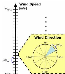
Fig. 9 Definition of the input wind profile for coherency analysis
