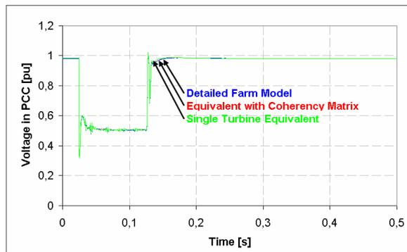
Fig. 17 Voltage in point of common coupling
