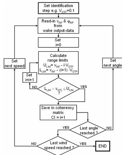
Fig. 11 Identification algorithm for construction of a coherency matrix
