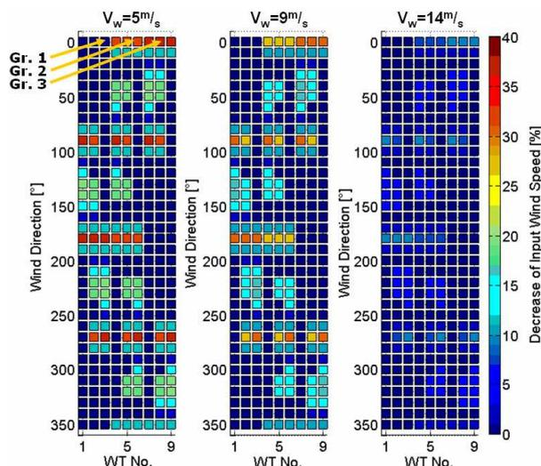
Fig. 10 Representation of the coherent wind turbines depending on the wind direction and wind speed
