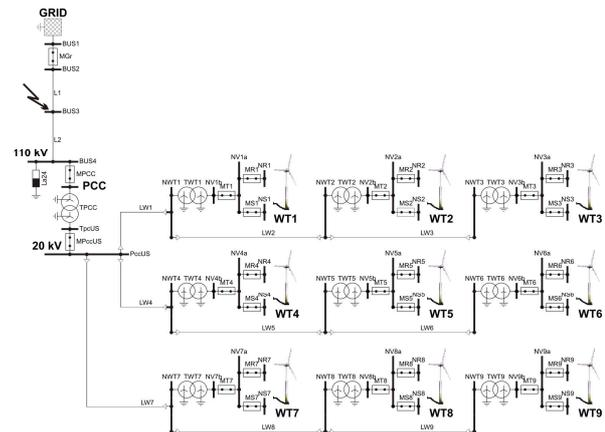
Fig. 13 Structure of the test system for dynamic simulation
