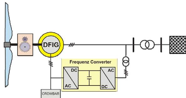
Fig. 1 Structure of the WT with DFIG
