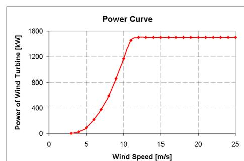
Fig. 12 Power curve of the variable speed WT
