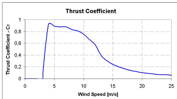
Fig. 5 Exemplary thrust characteristic of the wind turbine [12]
