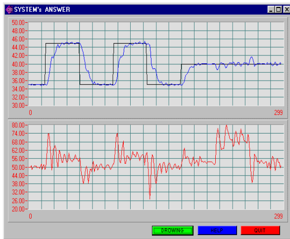
Fig. 6. Performances for P_0 operating point with (R_2, S_2, T_2) algorithm
