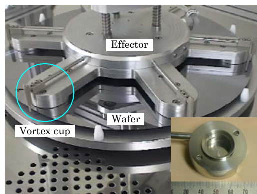
Fig. 2. Non-contact handling system by using air swirling flow
