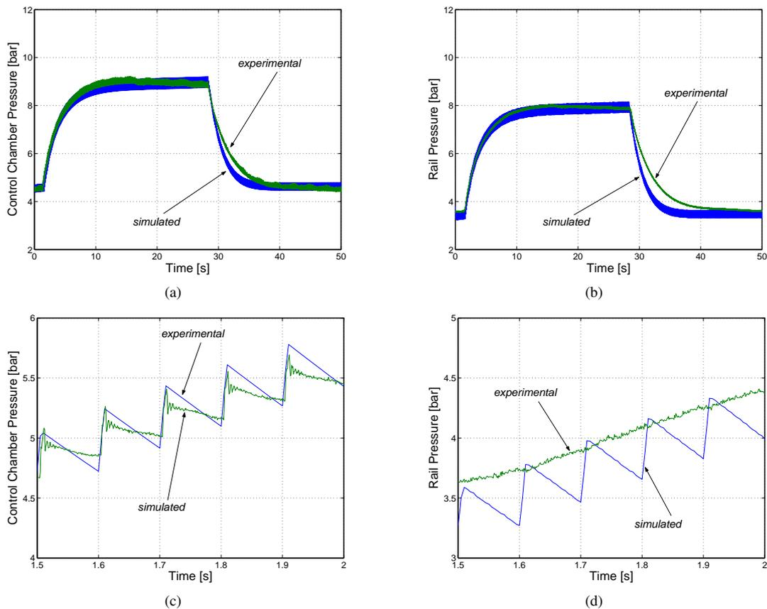
Fig. 3 State-space model and experimental results with duty cycle step variations and constant injectors driving signal; (a) control chamber pressure; (b) rail pressure; (c) detail on control chamber pressure; (d) detail on rail pressure.
