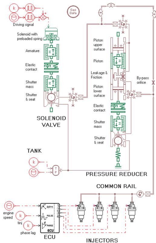
Fig. 2 AMESim model of the common rail CNG injection system
