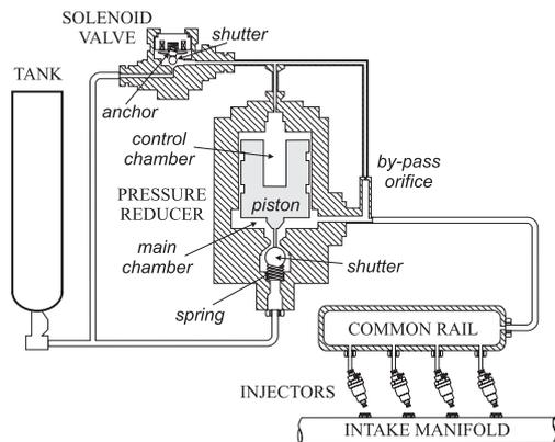
Fig. 1 Block scheme of the common rail CNG injection system
