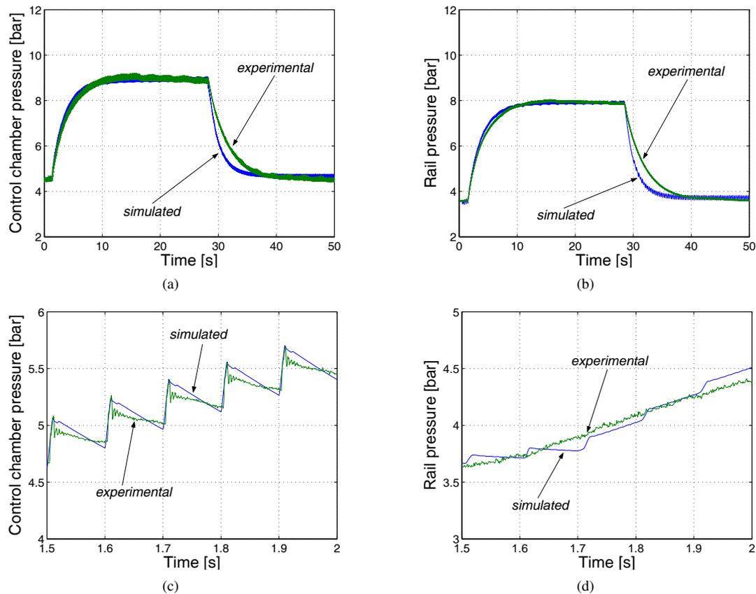
Fig. 4 AMESim model and experimental results with duty cycle step variations and constant injectors driving signal; (a) control chamber pressure; (b) rail pressure; (c) detail on control chamber pressure; (d) detail on rail pressure.
