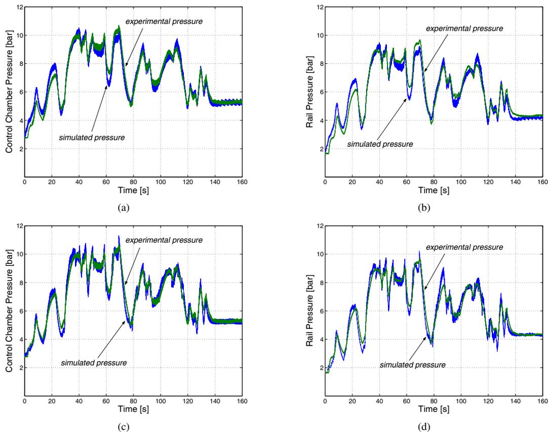
Fig. 6 Simulation and experimental results when varying duty cycle and engine speed, with a constant  $t_j = 3\text{ms}$ ; (a) State-space model control chamber pressure; (b) State-space model rail pressure; (c) AMESim model control chamber pressure; (d) AMESim model rail pressure.
