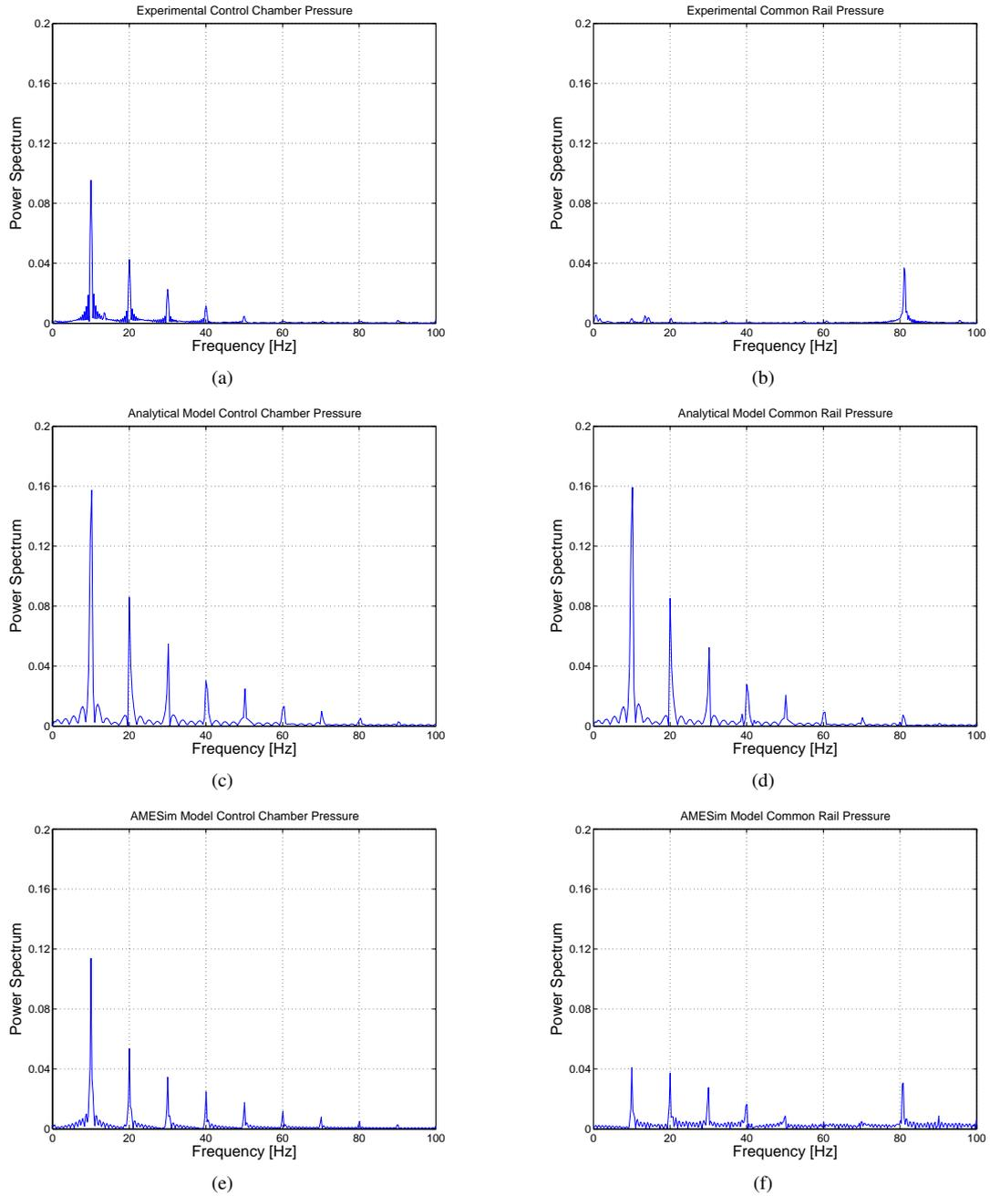
Fig. 5 Power spectrum of the control chamber and common rail pressures (a) Experimental control chamber pressure; (b) Experimental rail pressure; (c) State-space model control chamber pressure; (d) State-space model rail pressure; (e) AMESim model control chamber pressure; (f) AMESim model rail pressure;
