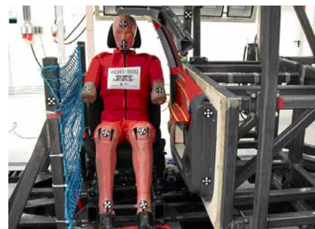
Fig. 8: MAGNA STEYR side impact test rig
