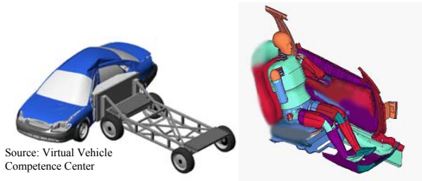
Fig. 4: Crash structural simulation vs. occupant simulation
