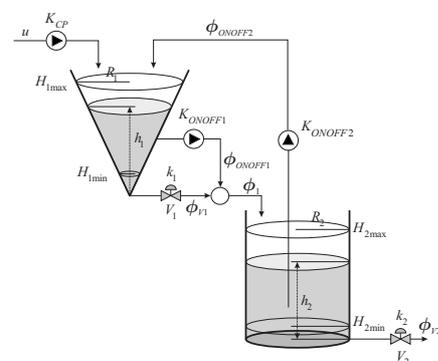
Fig. 1 The tank system plant.
