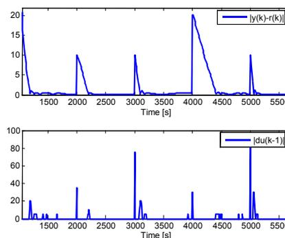
Fig.11. HFPC-EMO2. Tracking error  $|y(k)-r(k)|$ , control effort  $|\Delta u(k-1)|$  indexes.
