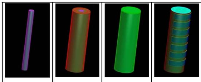
Fig. 1 Build up of the Lithium-Ion Battery simulation model including the electrolyte core, the wrapped electrode layers and the aluminum casing.
