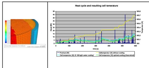
Fig. 4 Surface temperatures at the end of the cycle (left). Comparison of cell temperature for a case without cooling, with a realistic HTC and a cooling fluid temperature of 303 K and a case with the theoretical, optimal cooling (wall temperature 303K).
