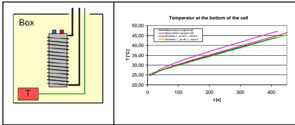
Fig. 2 Measurement set up (left), Results of the measurements/simulation for a heat flow volume of 18W (right). The simulations correlate with the measurements, especially the comparison with the original cell is good.
