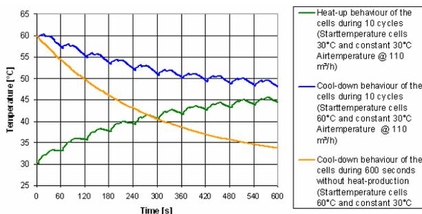
Fig. 9 Comparison of heat up and cool down behavior for a constant coolant temperature of 30°C and a constant mass flow.
