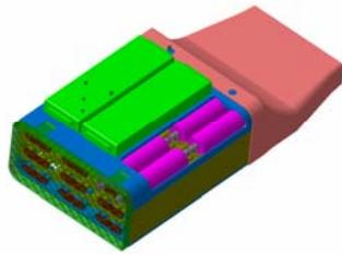
Fig. 1 The geometry consists of a channel, including brackets which secure the cells (pink) and nozzle with guiding vanes to route the cooling air to the outlet.
