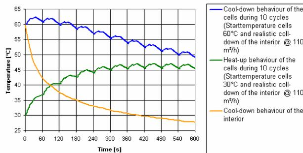
Fig. 10 Comparison of heat up and cool down behavior for a realistic cool down behavior of the passenger compartment.
