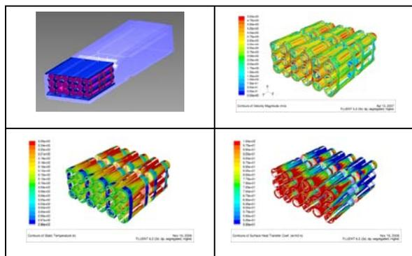
Fig. 2 Impressions of the flow and the heat up for 110 m<sup>3</sup>/h air volume flow and 10W/cell heat input
