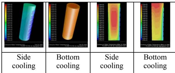
Fig. 3 State of stability temperatures for side and bottom cooling strategy. The resulting temperatures are better for side cooling.
