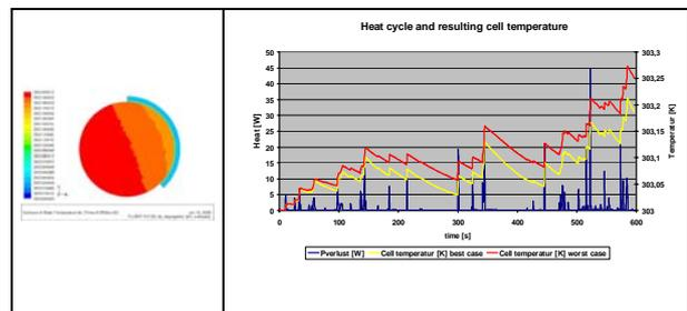
Fig. 5 Temperature in a plane cut Transient cell temperature for two different cooling fluid mass flows (right).
