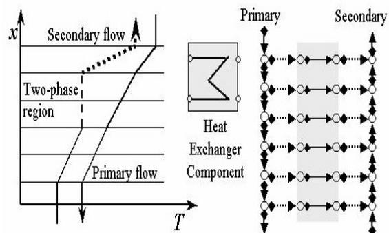
Figure 4. Heat exchanger nodalisation and relevant temperature distribution
