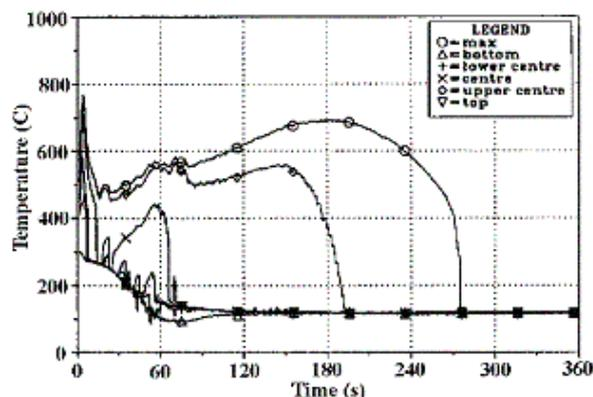
Figure 7. Fuel rod cladding temperature during loss of coolant accident
