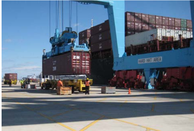
Fig. 3: Quay crane loading a container onto a chassis
