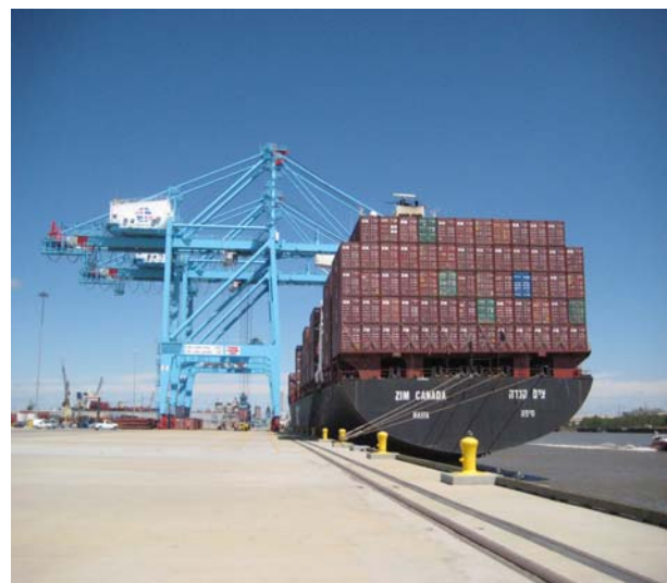
Fig. 2: Quay cranes unloading containers
